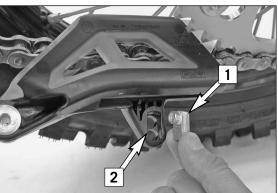
Loosen both screws on the chain guide and pull the chain guide off the swing arm. Turn the chain guide over, press out the retaining nut [1] and insert it in the other hole [2], turning the retaining nut around. Remount the chain guide and tighten the screws.
