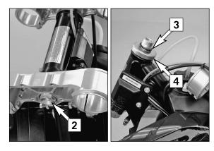
Loosen the clamp screws and take the fork legs out of the triple clamps. Loosen the collar screw **[2]** on the lower triple clamp 2 turns. Remove the blind screw **[1]** from the upper triple clamp, loosen the clamp
