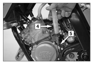
Fill the bleeder syringe [4] with a suitable fluid (see Technical Specifications - Engine). Remove the bleeder screw from the slave cylinder [5] and mount the bleeder syringe.
