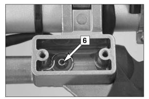
Press oil into the system until the fluid runs out of the hole [6] in the master cylinder without bubbles. Occasionally extract the fluid from the master cylinder reservoir to keep it from overflowing.
