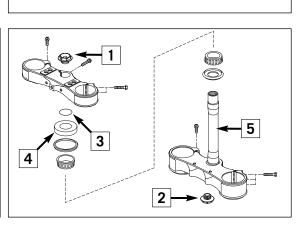
To adjust the offset, dismount the front wheel and remove the front wheel fender.
