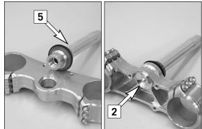
Remove the collar screw from the lower triple clamp and pull out the steering stem. Thoroughly clean all parts. Turn the steering stem 180° and insert it in the triple clamp. Apply Loctite 243 to the thread of the collar screw [2] and turn all the way in.
