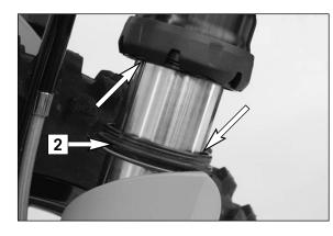
Thoroughly clean the dust boots, slide rings, outer tubes and fork tubes and oil generously with Universal oil spray (Motorex Joker 440) or engine oil. Press the dust boots into the outer tubes by hand. Position the fork protectors, mount the screws and torque to 10 Nm.
