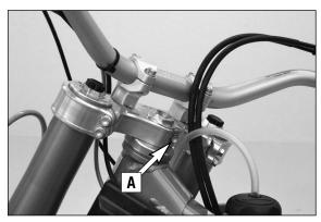
Mount the lower triple clamp, upper steering head bearing, protection ring, O-ring, upper triple clamp and the blind screw.
