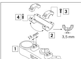
For this purpose, remove screws **[3]** of the handlebar clamps and screws **[4]** of the handlebar support. Position the handlebar support, and tighten screws **[4]** to 40 Nm (30 ft.lbs). Mount the handlebar and handlebar clamps, and tighten screws **[3]** to 20 Nm (15 ft.lbs). The gap between the handlebar support and the handlebar clamps should be the same size in the front and in the rear.
