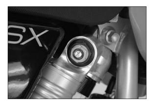
**Damping action during compression of shock absorber (SX)** The shock absorber on the SX models can synchronize the compression damping in the low and high-speed range separately (Dual Compression Control).
