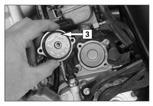
Put the motorcycle on its side and fill the oil filter housing about halfway with engine oil. Fill oil filter with oil, place the oil filter in the filter box. Grease the O-ring [3] of the oil filter cover and mount the cover. Mount the screws and tighten them to 6 Nm.
