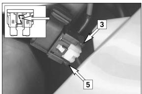
The starter relay also contains a (10 amp) spare fuse [5].
