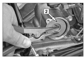
Using circlip pliers, pull the oil-filter insert [2] out of the housing. Clean the oil filter cover, the sealing surface of the O-ring and the engine casing. Check the O-ring of the oil filter covers for damage and, if necessary, replace it
