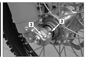
To install the front wheel, lift it into the fork, position and mount the axle shaft. Mount the collar nut [2], tighten the clamping screws [3] on the right fork leg axle passage to prevent the axle shaft from turning and tighten the collar nut to 40 Nm (30ft.lb).
