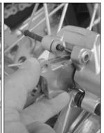
Insert the left brake pad into the brake caliper and secure it with the bolt. Insert the right brake pad and push the bolt [5] into the brake caliper up to the stop. Reattach clips [4].
