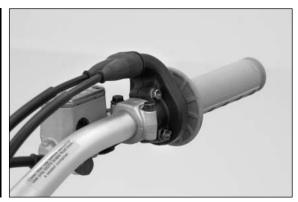
Mount the front wheel fender and tighten the screws to 10 Nm. Mount the hand brake cylinder and tighten the screws to 10 Nm. Mount the starting number plate.
