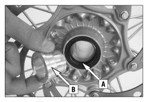
Before remounting the front wheel, clean and grease the shaft seal rings [A] and the bearing surface [B] of the distance bushings and mount the distance bushing
