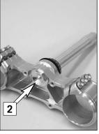
Remove the collar screw from the lower triple clamp and pull out the steering stem. Thoroughly clean all parts. Turn the steering stem  $180^{\circ}$  and insert it in the triple clamp, tighten the collar screw all the way to the stop. Grease the steering head bearing and sealing elements.
