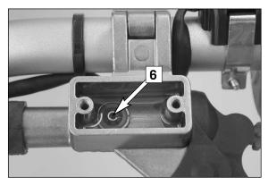
Press oil into the system until the oil runs out of the hole [6] in the master cylinder without bubbles. Occasionally extract the oil from the master cylinder reservoir to keep it from overflowing.
