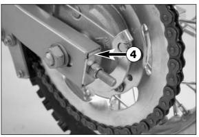
To mount the wheel reverse the procedure described above. Always hook the brake backing plate into the swing arm support. Before tightening the hexagon nut of the wheel spindle, ensure that the supporting plates ② are resting against the swing arm. Additionally, check that the rear wheel is aligned with the front wheel. Tighten the hexagon nut to 30 Nm.
