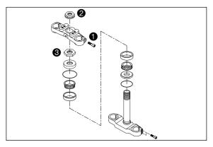
At least once a year, the steering head bearings should be smeared with waterproof grease (Shell Advance Grease).
