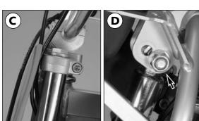
Figures C and D show the fork and shock absorber positions for a high seat position. Fork tubes are plane with top of upper fork stabilizer. (Screw cap (Aluminium) protrudes from the top of the upper fork stabilizer)
