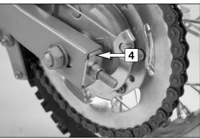
To mount the wheel reverse the procedure described above. Always hook the brake backing plate into the swing arm support. Before tightening the hexagon nut of the wheel spindle, ensure that the supporting plates [4] are resting against the swing arm. Additionally, check that the rear wheel is aligned with the front wheel. Tighten the hexagon nut to 40 Nm.
