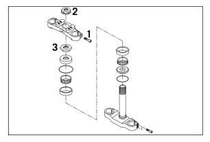
At least once a year, the steering head bearings should be smeared with water-proof grease (Motorex Long Term 2000).
