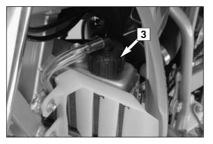
A mixture of 50 % antifreeze and 50 % distilled water is used as the cooling liquid. How-ever, the antifreeze protection must be at least -25° C (-13° F). This mixture offers antifreeze protection but also good corrosion protection and should therefore not be replaced by pure water.
