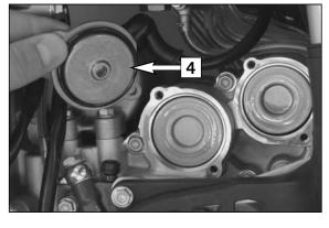
Put the motorcycle on its side and fill the oil filter housings about halfway with engine oil. Fill oil filter with oil, place the long oil filter in the front and the short filter in the back of the filter box.
