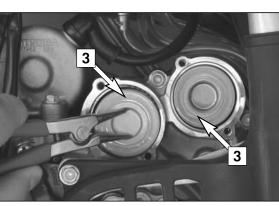
Using circlip pliers, pull the oil-filter inserts **[3]** out of the housing. Clean the oil filter cover, the sealing surfaces of the O-rings and the engine casing. Check the O-rings of the oil filter covers for damage and, if necessary, replace them.
