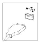
**1.5.2** Connect the mouse cable to the appropriate mouse port (USB port). (Not all models are equipped with a mouse.)
