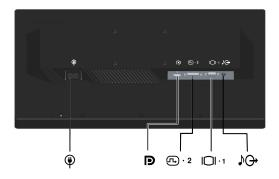
3. Connect one end of the analog signal cable to the monitor VGA connector and the other end to the computer.
