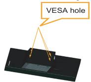
Step 5: Attach the LCD display to the wall, following the instructions in the wall-mounting kit.
