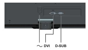
3. Connect one end of the analog signal cable to the monitor VGA connector and the other end to the computer.
