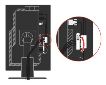
Wrap the Cable Wrapper around the cables.
