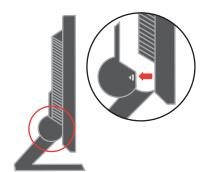
This allows access to the screws that attach the stand to the monitor.
