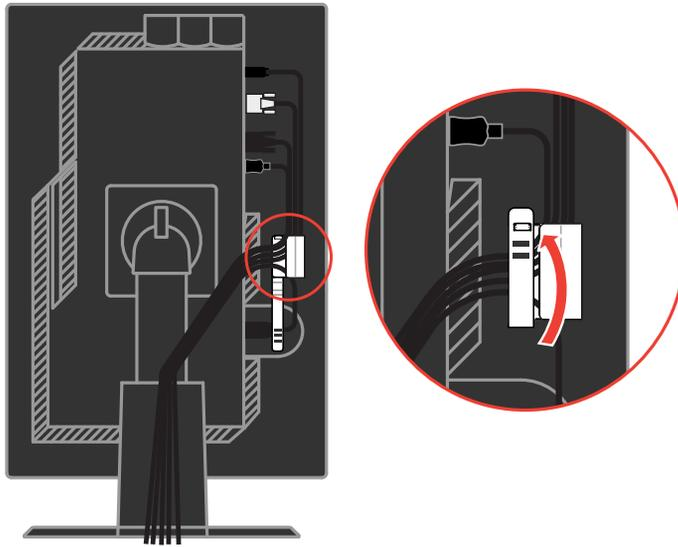
Wrap the Cable Wrapper around the cables.
