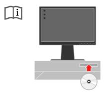
To optimize your monitor image, if using the analog cable, press the Automatic Image Setup key. Automatic image setup requires that the monitor is warmed up for at least 15 minutes. This is not required if you are using the DVI cable.
