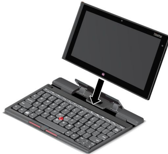
Figure 8. Installing the tablet into the Bluetooth keyboard
