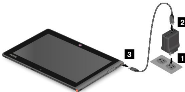
Figure 4. Connecting the ac adapter with the tablet
