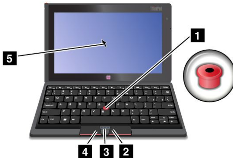
Figure 9. Using the optical TrackPoint
