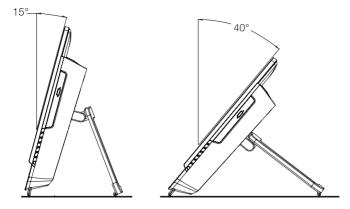
Use the stand to position the display to your preference. It can be rotated between  $15^{\circ}$  and  $40^{\circ}$  from the vertical.
