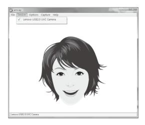
3) Confirm that Devices → Lenovo USB2.0 UVC Camera has been checked. If there are other devices in this option, do not check them. Only choose the "Lenovo USB2.0 UVC Camera" device, and the window should display the camera image. An image, which is caught by Lenovo PC camera, will be displayed in the video capture window. Adjust the position and pitch angle of the camera to ensure the whole face is displayed in the video capture window.
