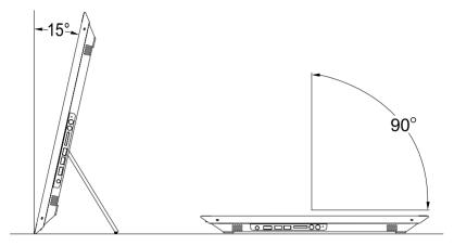
Use the stand to position the display to your preference. It can be rotated between  $15^{\circ}$  and  $90^{\circ}$  from the vertical.
