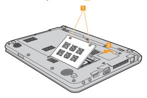
6 Press outwards on the latches on both edges of the socket at the same time, remove the SO-DIMM. Be sure to save the old SO-DIMM for future use.
