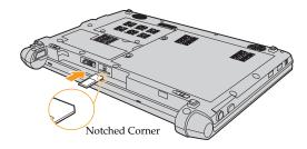
**6** Put the battery back in place, turn the computer over again, and reconnect the cables.
