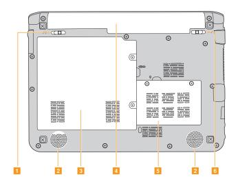
Battery latch -The manual battery latch is used to keep the battery pack secured in place. manual Speakers The stereo speakers provide rich and powerful sound. PCI Mini **ExpressCard** slot/hard disk drive (HDD) compartment **Battery pack** For details, see "Using AC adapter and battery" on page 11. Memory compartment Battery latch -The spring-loaded battery latch keeps the battery pack secured in place. spring loaded
