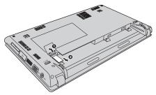
**(a)** Put the battery back in place. Turn the computer over and reconnect the cables.
