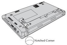
**6** Put the battery back in place. Turn the computer over and reconnect the cables.
