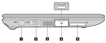
1 AC power Connect the AC adapter here.
