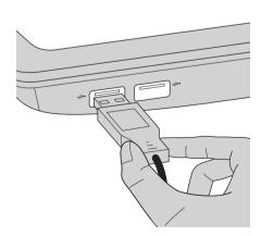
The first time you plug a USB device into a particular USB port on your computer, Windows automatically installs a driver for that device. After the
