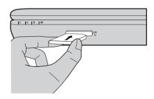
**2** Gently slide the memory card into the card slot until it reaches the end.
