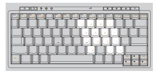
**Note:** The **1** indicator will light on if the numeric keypad is enabled.
