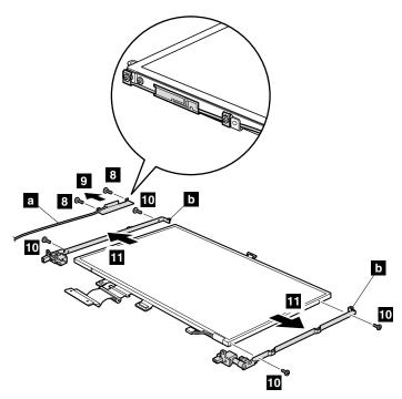
In steps 8 and 9, remove the wireless LAN 3rd antenna (a) from the left hinge.
