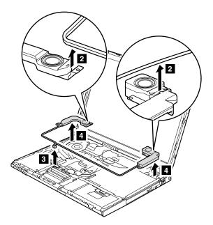
**When installing:** Make sure that the speaker connector is attached firmly, and the cables are routed as in this figure.
