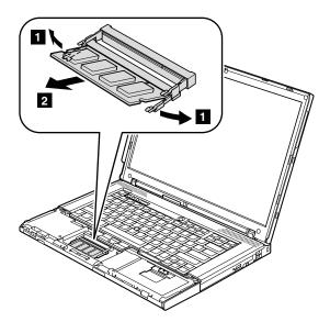
When installing: Insert the notched end of the DIMM into the socket. Press the DIMM firmly, and pivot it until it snaps into the place. Make sure that it is firmly fixed in the slot and does not move easily.
