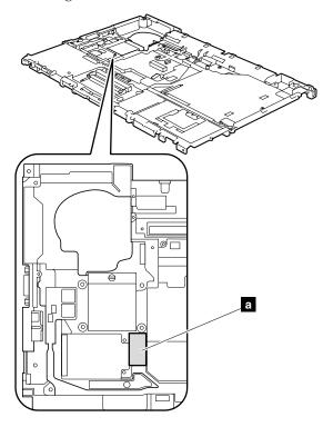
2. For the models with Sierra Wireless EV-DO Wireless WAN Mini PCI Express Adapter, you need to attach the shield sheet that is shipped with new structure frame. Peel off the covering film of the adhesive tape on bottom side of the shield sheet, and paste it on the new structure frame as shown in this figure.
