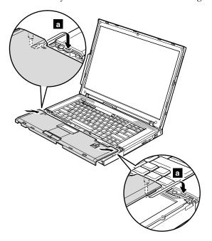
3. Align the front side of the palm rest to the frame, and press the front edge to latch the palm rest to the frame as shown in this figure.
