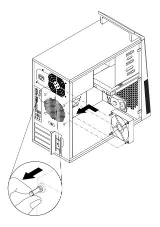
Figure 44. Installing the rear fan assembly
