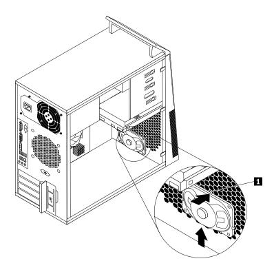
Figure 46. Removing the old internal speaker
