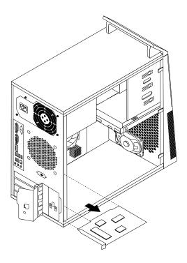
Figure 12. Removing a PCI card
