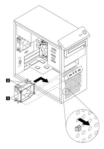
Figure 42. Installing the front fan assembly
