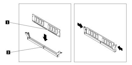
Figure 16. Installing a memory module
