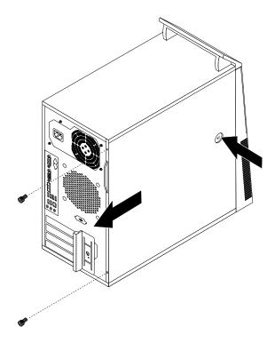
Figure 9. Removing the computer cover
