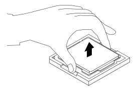
Figure 33. Removing the microprocessor
