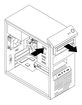
Figure 17. Removing the optical drive
