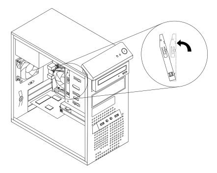
Figure 21. Removing the card reader retainer
