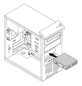
Figure 23. Installing the card reader
