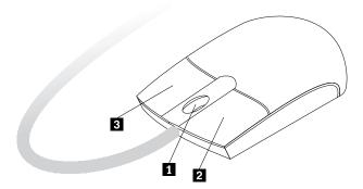
Use the wheel to control the scrolling action of the mouse. The direction in which you rotate the wheel controls the direction of the scrolling action.
