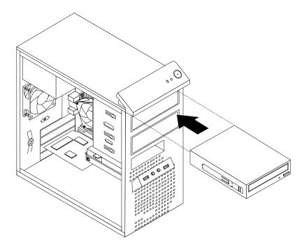
Figure 19. Installing the optical drive
