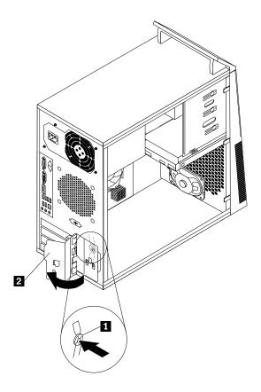
Figure 11. Opening the PCI card latch
