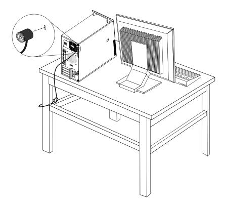
Figure 8. Integrated cable lock
