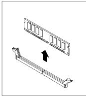
Figure 14. Removing a memory module
