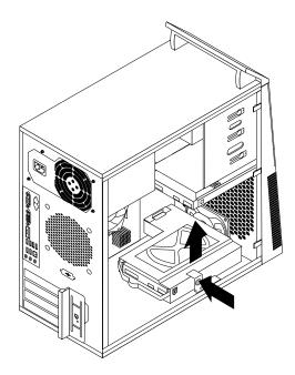
Figure 38. Removing the secondary hard disk drive
