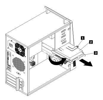
Figure 35. Removing the primary hard disk drive
