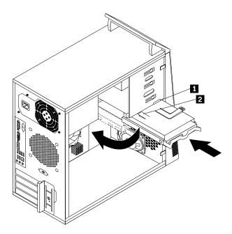
Figure 37. Installing the primary hard disk drive
