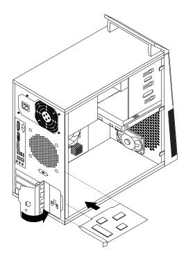
Figure 13. Installing a PCI card
