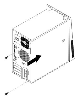
Figure 49. Reinstalling the computer cover
