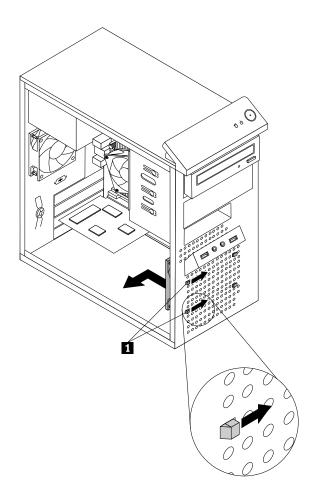
Figure 41. Removing the front fan assembly
