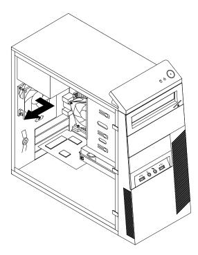
Figure 43. Removing the rear fan assembly
