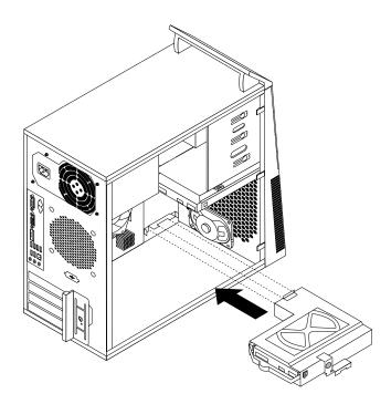
Figure 40. Installing the secondary hard disk drive
