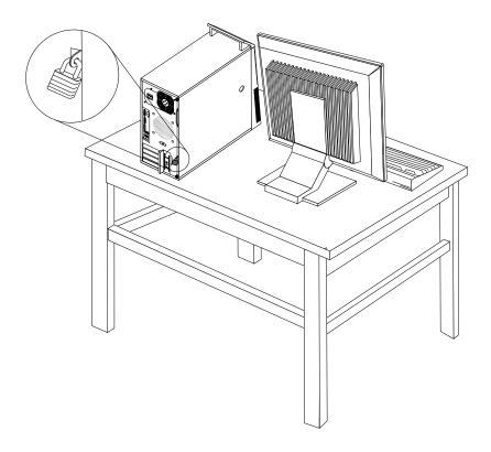
Figure 7. Installing a padlock
