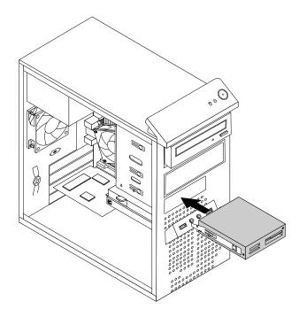
Figure 27. Installing the card reader
