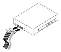
Figure 20. Connecting the optical drive
