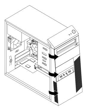
Figure 10. Removing the front bezel
