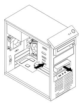
Figure 25. Removing the card reader
