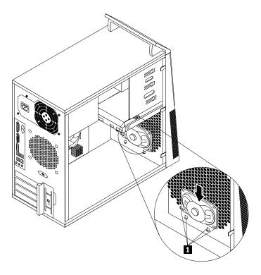
Figure 47. Installing a new internal speaker
