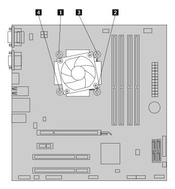
Figure 31. Removing the heat sink and fan assembly
