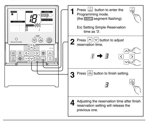
\* If the indoor is ON, we can make the reservation for turning OFF. In reserve, if the indoor is OFF, we can set the timer for turning ON. The reservation time is from 1 to 7 hours.
