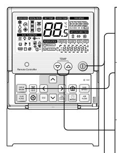
Press the Run/Stop button on the control part of the remote controller to start the operation.
