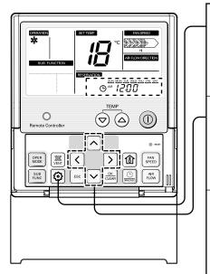
Keep pressing button for 4 secs to enter Setting current time mode.
