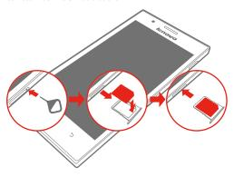
Step 1. Insert the SIM eject tool into the hole on the SIM card tray.
