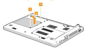
**6** Remove the frame fixing screws.
