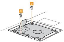
**6** Pull the tab in the direction shown by arrow.
