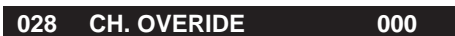
After Master TV setup has been completed, set Installer menu item 028 Ch Override to 000.
