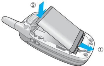
5. Press the battery until it clicks into place. Make sure that the battery is properly installed before switching the phone on.
