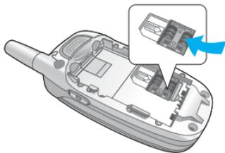
4. Place the battery so that the tabs on the end align with the slots at the bottom of the phone.
