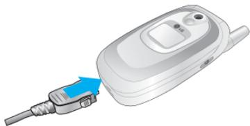
**Warning** You must unplug the adapter before removing the battery from the phone during charging; otherwise, the phone could be damaged.
