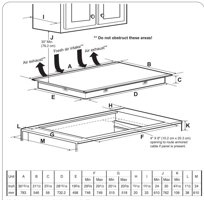
All dimensions are stated in inches and millimeters (mm).
