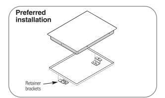
NOTE: The retainer brackets MUST be installed to meet local codes or, in their absence, with the National Electrical Code ANSI/NFPA No. 70, latest edition.
