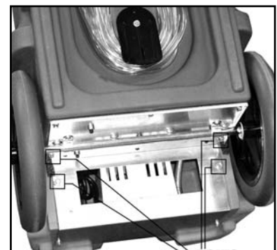
Pump removal, location of 4 bolts
