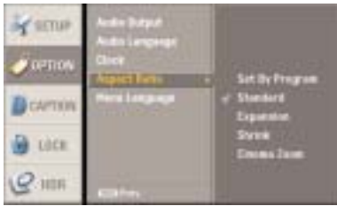
Menu for a wide (16:9) aspect ratio at 480i or 480p mode output format.
