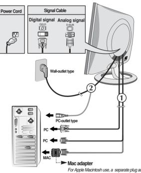
For Apple Macintosh use, a separate plug adapter is needed to change the 15 pin high density (3 row) D-sub VGA connector on the supplied cable to a 15 pin 2 row connector.
