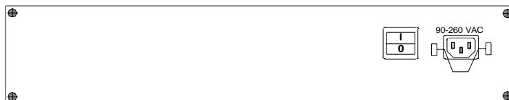
Figure 6-9. AC Power Distribution Panel—Front View
