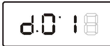
Figure 4-1 Example of the front panel display for the diagnostic main menu
