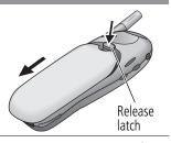
2 Pull down the battery release latch.
