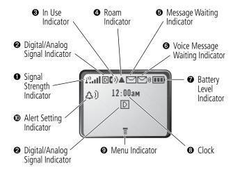
**O** Signal Strength Indicator Shows the strength of your phone's connection with the network.
