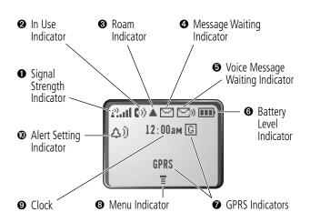
• Signal Strength Indicator Shows the strength of your phone's connection with the network.
