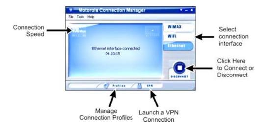
This interface allows you to connect to an Ethernet-based (wired) network utilizing the same credentials (where applicable) utilized for connections to WiFi hotspots.
