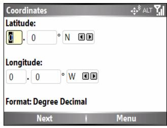
Press the menu button to change the way you view the coordinates. There are three options: Degree Decimal, Degree Minute Second, or Degree Minute Decimal.
