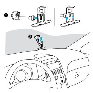
**Note:** You can also affix suction cup to the dashboard using the included circular disc (not shown). To do this, affix circular disc to your dash or center console, then attach the suction cup on the extension arm to the disc.
