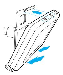
4 Using both hands, adjust extension arm for optimal viewing off your MOTONAV TN30.
