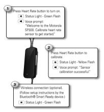
**Note:** Motorola SF500 is a Bluetooth® Smart heart rate monitor. Wireless connection to a Bluetooth® Smart Ready device enables transmission of heart rate data. Check your phone or device manual for Bluetooth compatibility.
