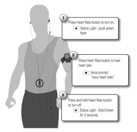
**Note:** The heart rate monitor can be used at anytime. It does not require the headphones to be plugged in to a device.
