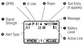
• Signal Strength Indicator Indicates the strength of your phone's connection with the network.
