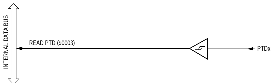
Figure 15-12. Port D Input Circuit
