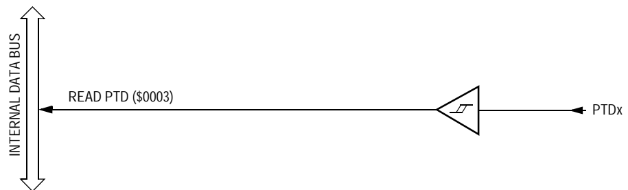
Figure 15-12. Port D Input Circuit
