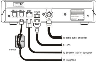
If you already have a TV connected to the cable outlet, you will need to use a 5-900 MHz splitter. Connect the coaxial cable as shown below:
