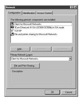
The CG3500 contains all necessary software. You don't need to configure the CG3500, but you must configure your computer for TCP/IP and check for an IP address. Your service provider may provide additional instructions for setting up your computer. The following basic instructions are for Windows $^{\text{TM}}$  95 or Windows 98. If you are using a different operating system, refer to that user guide.
