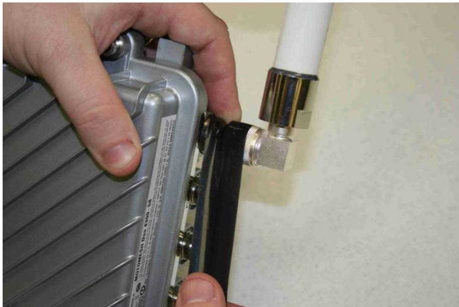
Figure 4-14 Finish wrapping the tape around the antenna base
