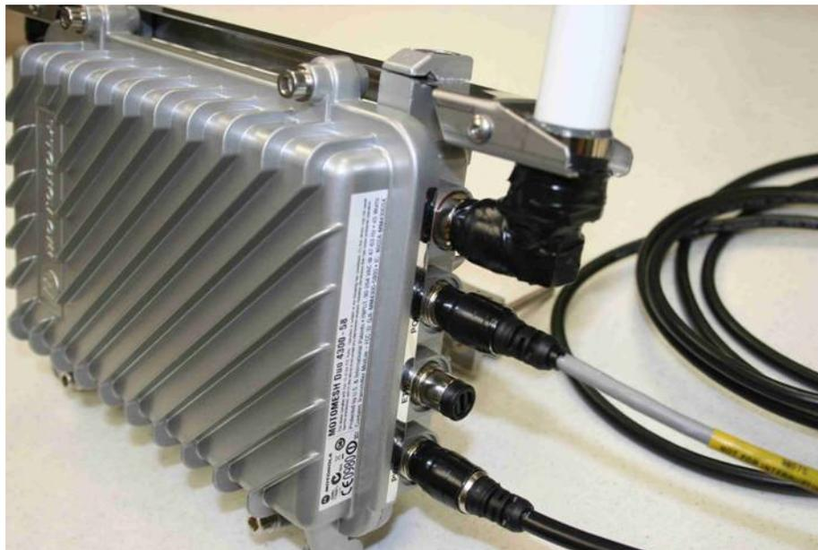
The majority of your MOTOMESH Duo devices will only have a power connection (unless the device is an IAP). If the MWR is going to be used to power a PoE capable device (such as an IP camera) then add the white personality plug to the select port (standards based 802.3af PoE) and connect the Ethernet cable to the POE OPT port.
