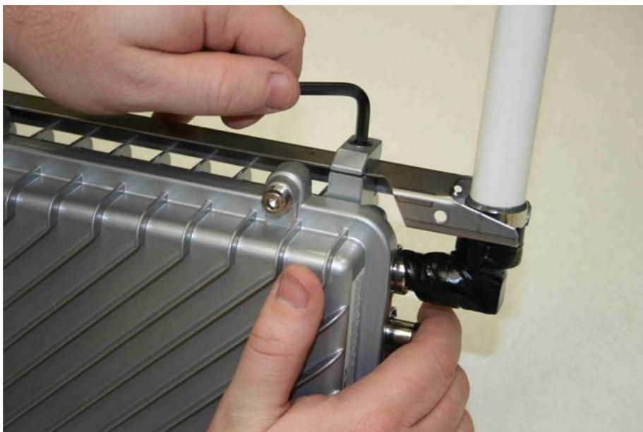
Figure 4-18 Tighten the bracket screws
