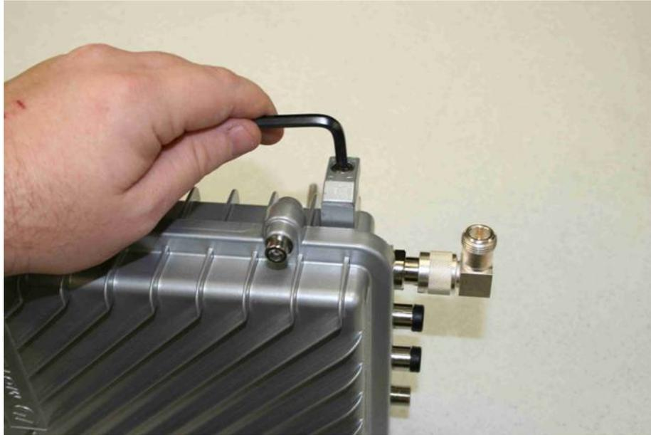
If using the 2.4 GHz down tilt antenna (which has a larger base) angle the bracket to fit around the base of the antenna.
