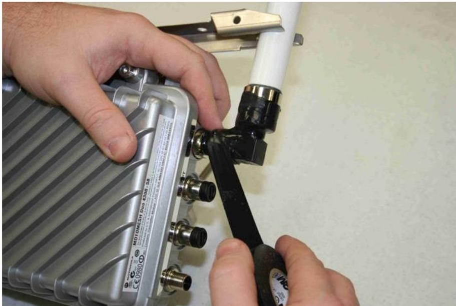
Figure 4-17 Tighten the antenna bracket
