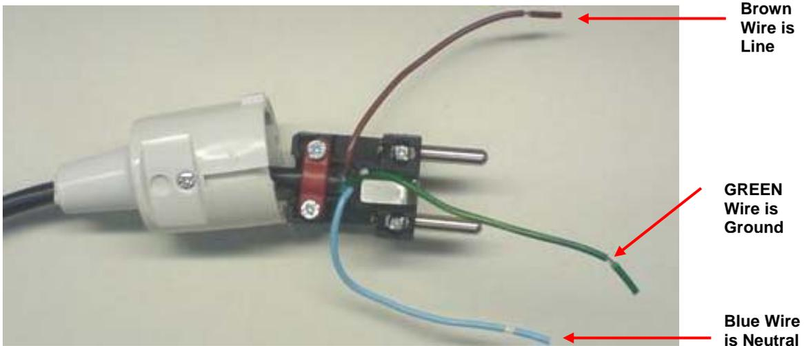
6. Loosen the Neutral, Line, and Earth Ground Screws.
