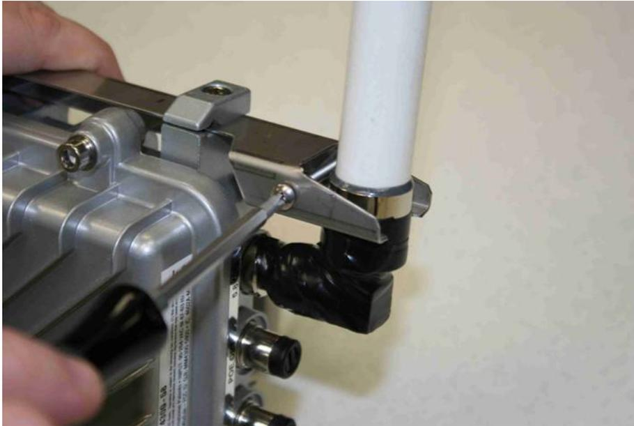
If your MOTOMESH Duo device is going to be used as an IAP remove the protective cap on the POE OPT Ethernet port. The POE OPT port is configured by default to be used as the backhaul port. Note that this port is NOT powered unless a personality plug is attached to the select port. Please see Chapter 3 for more information. Note that the Ethernet cable and port are keyed.
