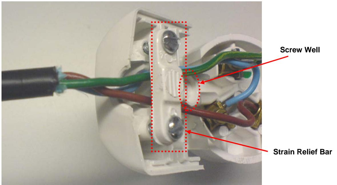
4. Press the wire base against the plug so that the wires are pulled through and the cable fits snugly at the base of the plug. Tighten the two Strain Relief Screws to lock the cable in place. See the graphic below for an example of the desired effect.
