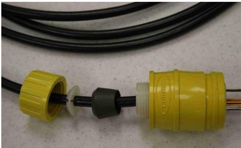
**Figure 9-7 Tighten plug**
