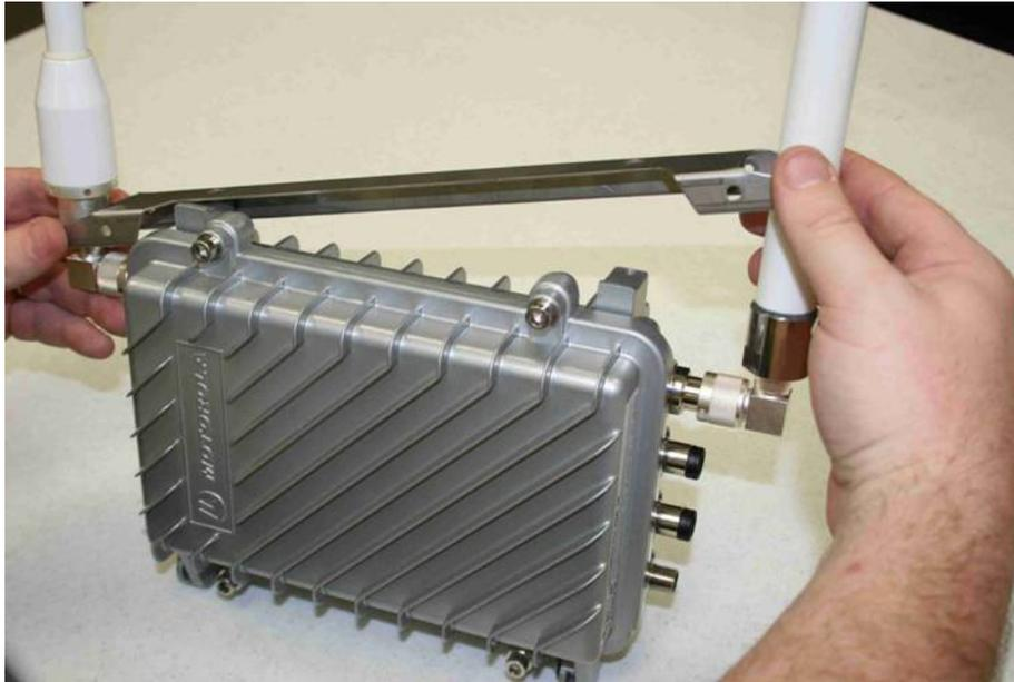
Carefully tighten both antennas. Do not over tighten. Never tighten the antennas by the plastic radome.
