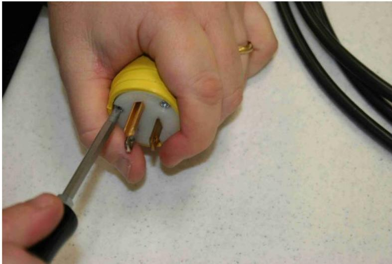
5. Insert Plug Terminal into Connector Body and tighten.
