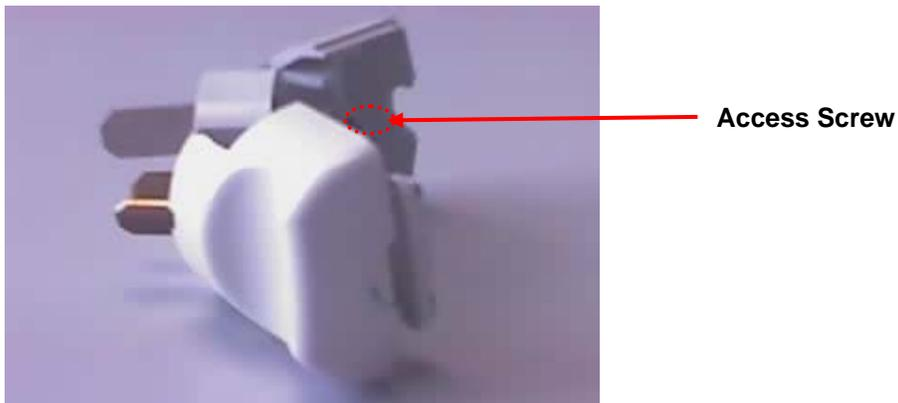
3. Place the plug down with its contents open and facing up. The *Strain Relief* section of the plug should be on the left hand side, as shown in the graphic below.
