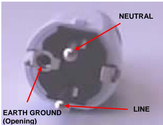
**Figure 9-10 European Power Connector Side View**
