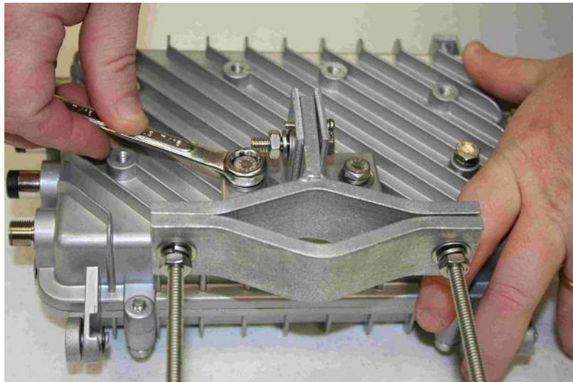
Loosen the pivot screw so the bracket is free to rotate.
