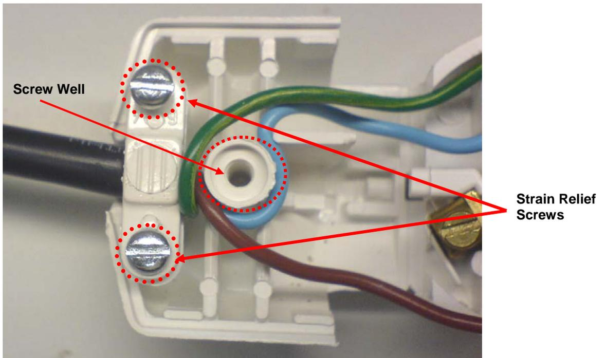
5. Attach the cable wires to the terminal plug in the following way.
