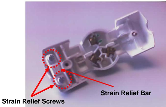
3. Place the three wires under the *Strain Relief Bar* and pull through. Allow the **Blue** and **Green Wire** to pull through on the left side of the *Screw Well* and the **Brown** Wire to pull through on the right hand side of the *Screw Well*.
