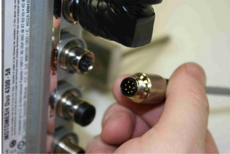
Figure 4-21 Connecting the power cable
