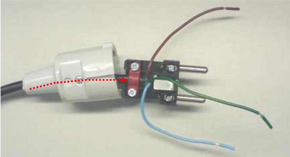
3. Press the wire base *under* the *Strain Relief Bar* so that the main cable is *not* visible on the other side of it.
