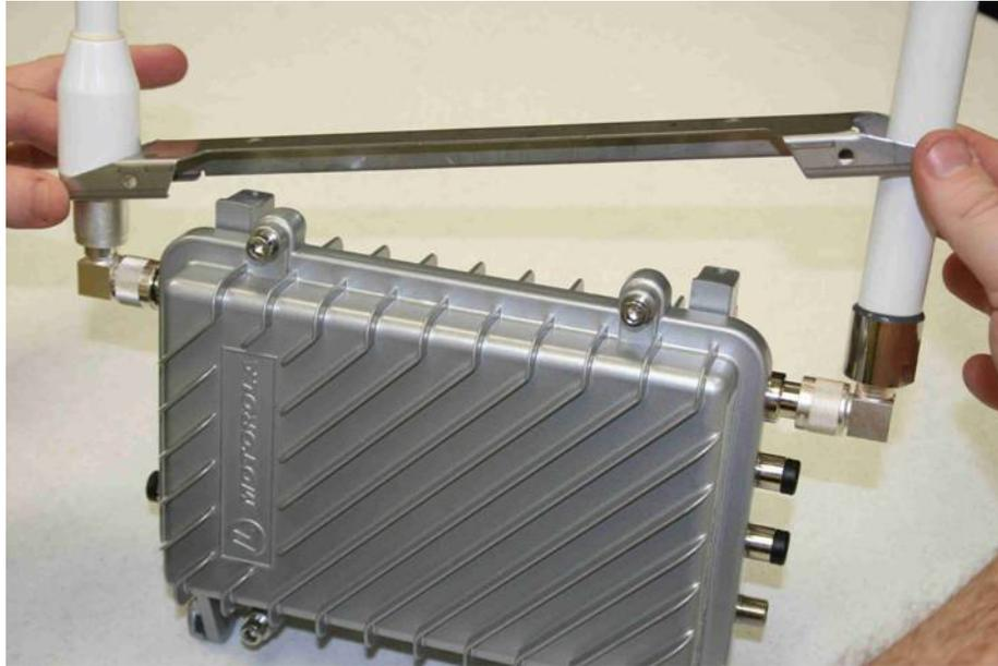
Stretch the weatherproof tape around the antenna connector
