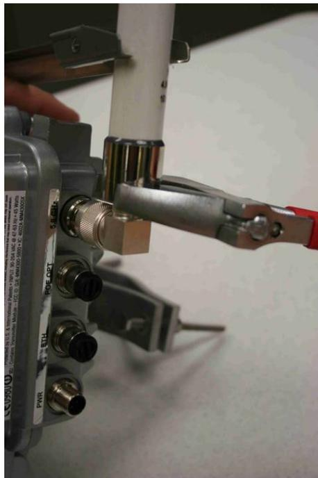
Slide the bracket up to make additional room to apply the weatherproof tape.
