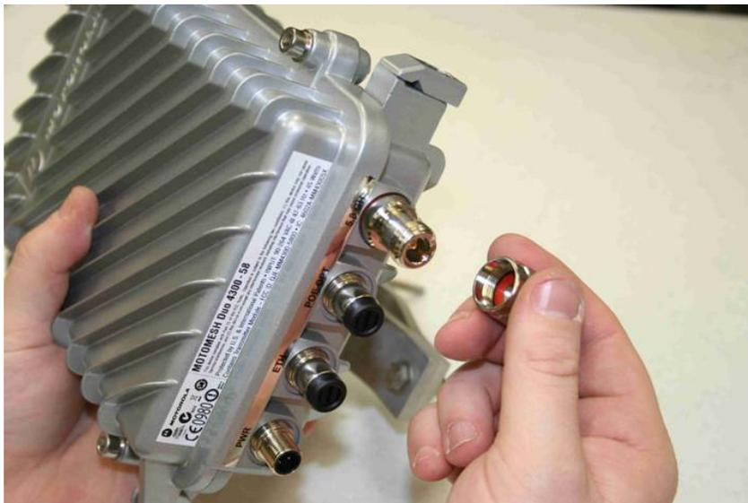
Attach the right angle antenna connectors.
