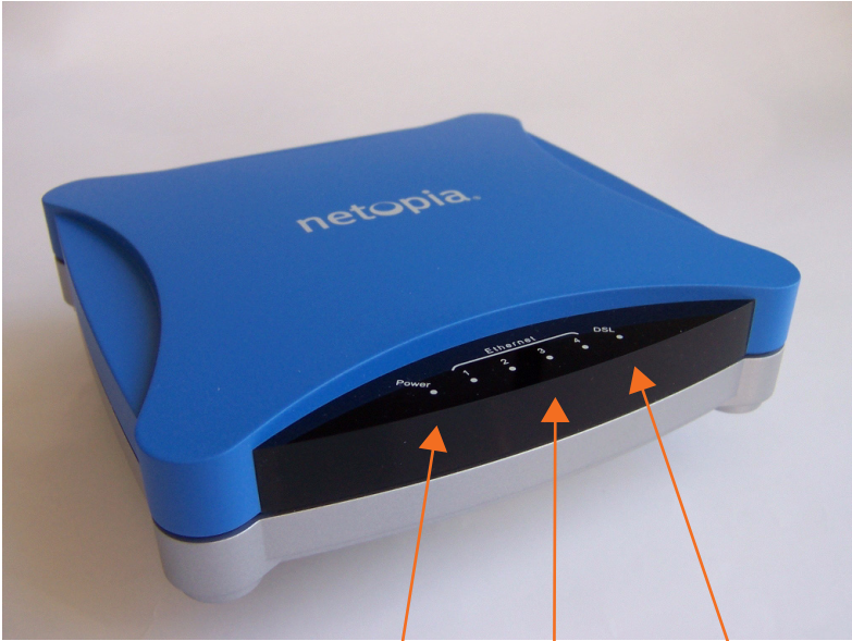
Power Ethernet 1, 2, 3, 4 DSL
