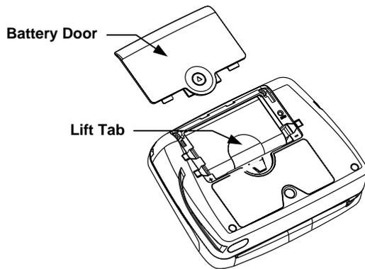
4. Using the white lift tab, lift the battery from the battery compartment.
