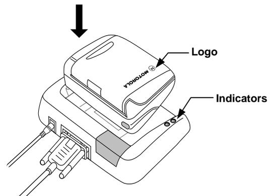
5. Press the pager down into the charger until an audible click is heard. The red LED indicator light means the battery is charging.
