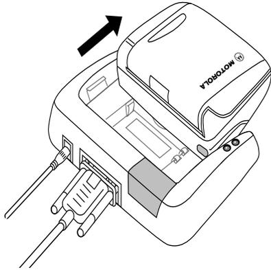
7. Remove the round transformer connector from the back of the charger, then remove the plug from the power supply.
