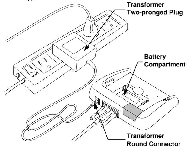
2. Insert the transformer's two-pronged plug into any standard 120 Vac power supply outlet.
