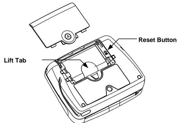
4. Using a pen or other small pointed object, press the reset button.
