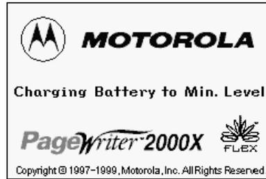
The charging indicator will move across the screen from left to right, until the screen is completed covered. This process usually takes about 10 minutes.
