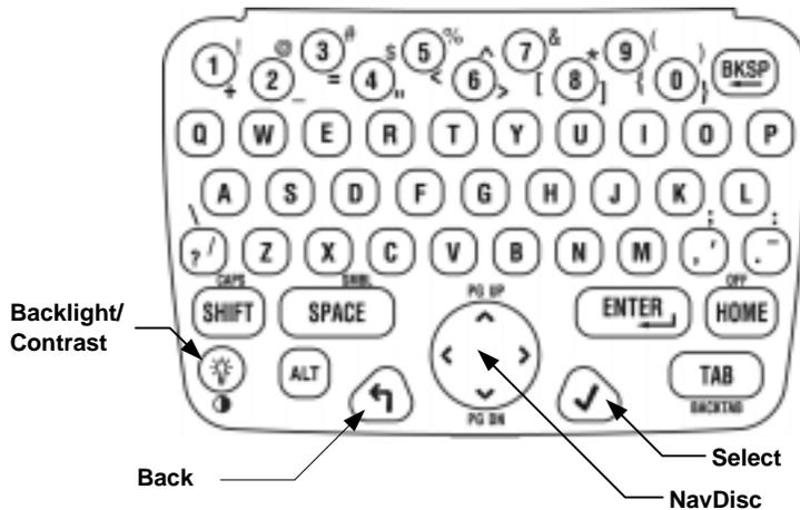
The PageWriter 2000X smart pager comes with a QWERTY keyboard. Special control keys and key combinations provide the following functions.
