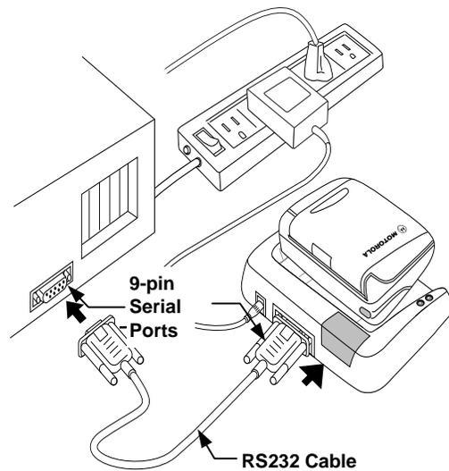
3. Insert the transformer's round connector into the back of the charger.
